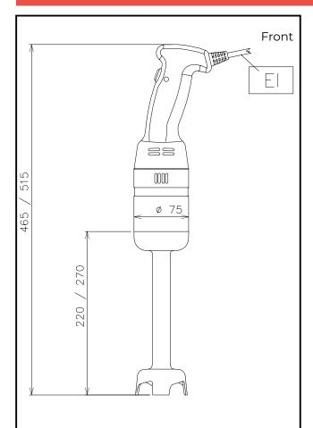
Electric Supply voltage: 230 V/1N ph/50 Hz Electrical power, max: 0.25 kW **Total Watts:** 0.25 kW
